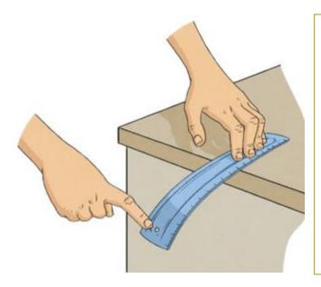
Experiment making a ruler vibrate over the edge of a desk.
